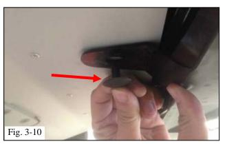
(h) Obtain the three black plastic ratchet fasteners from the hardware bag. Install/push them through the plastic bumper tabs into the holes on the skidplate (3 places) (Fig. 3-10).
